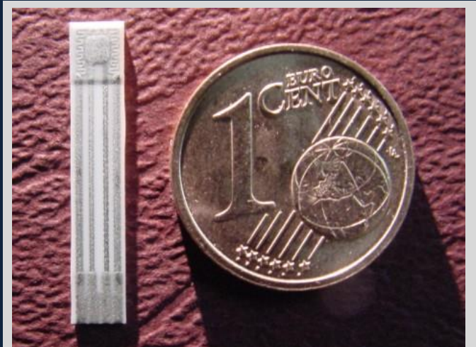
The miniaturisation of the ceramic sensor elements, which was essential for their use in aerospace activities, led to a variety of terrestrial uses. To meet the standards set by ESCUBE's customers, new manufacturing procedures are used in producing the sensor elements. This guarantees a high quality product also available in larger quantities.
